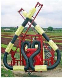
hydraulically, to provide auick and comfortable height adjustment and folding of the boom. This can be done either via the joystick or directly with the hydraulic lever in the tractor.
