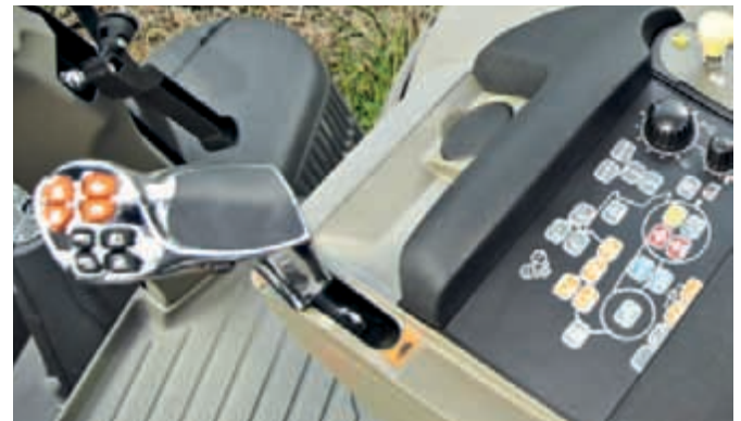
Multicontroller™ allows gear change without activating the clutch.
