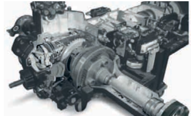
Six-speed Semi-Powershift and Full Powershift transmission maximize efficiency and increase productivity in the field and on the road.
