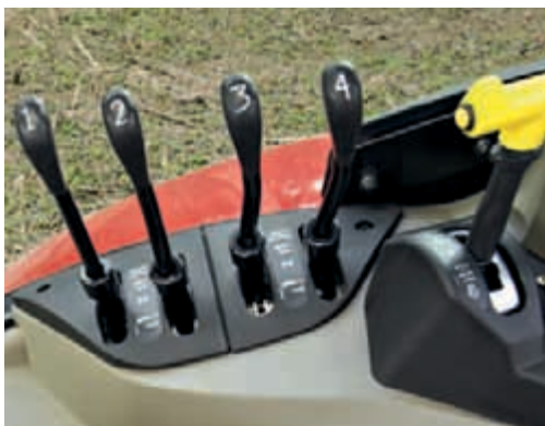
Up to four mechanical remote valves available as alternative to electronic remotes.
