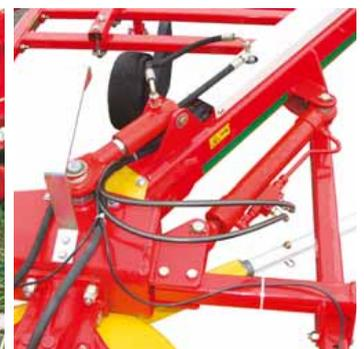
Hydraulic working width adjustment
