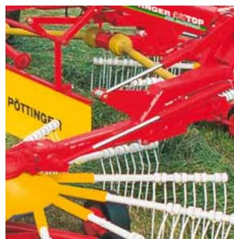
Hydraulic working width and swath width adjustment
