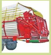
A uniformly distributed blanket of forage is essential for perfect compression. The discharge system features three beaters to protect the machine and make life easier for the driver. A twobeater system is also available for working in clamps.
