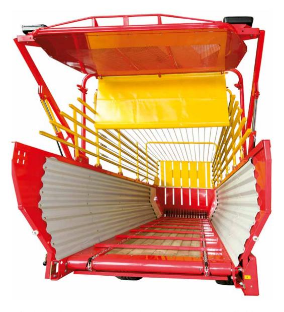
■ Opening the tailgate conveniently from the driver's seat is a standard feature. The full cross-section of the tailgate is open to allow rapid and unrestricted unloading.
