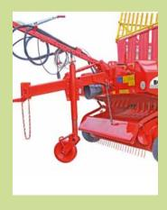
The hydraulically hinged drawbar (optional) with ground clearance of 23.62" / 600 mm under the pickup guarantees unobstructed driving over the clamp and on undulating ground.
