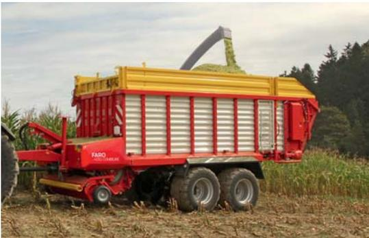
With the new **FARO 5010** and **FARO 4010 COMBILINE**, **PÖTTINGER** offers you new models in the medium-capacity loader wagon segment ranging between **90 and 150 hp**. The 31-knive knife bank and powerful rotor drive for higher capacity make the new FARO a high-performance loader wagon. The FARO 4010 COMBILINE can also be used as a harvest transport wagon, turning it into a cost-effective all-rounder.
