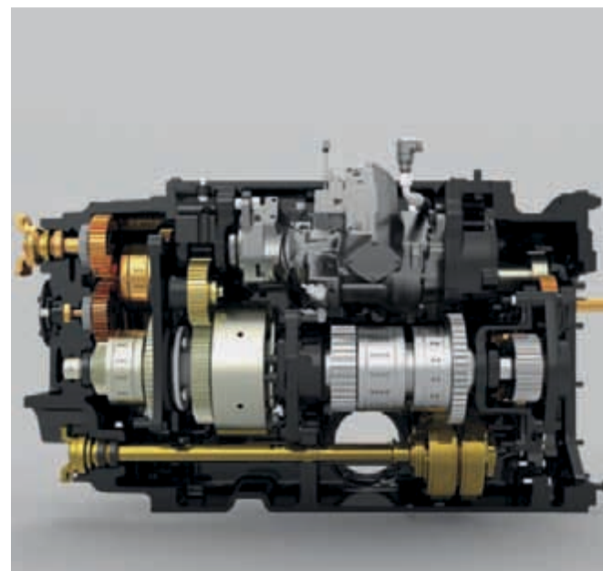
CVX transmission - stepless drive between 0-50kph
