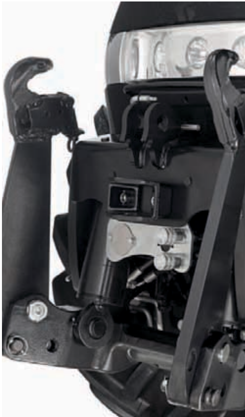
Seamlessly integrated Front Linkage with a lifting power of 5,000kg
