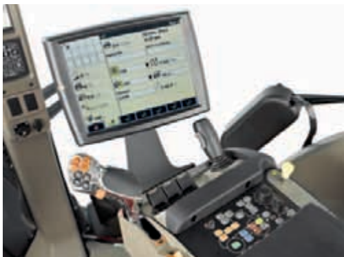
Multicontroller Armrest: Same Operator Environment from 100 to 620HP
