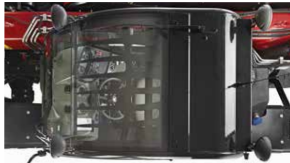
Safety is ensured through the structure's ROPS/FOPS status.
