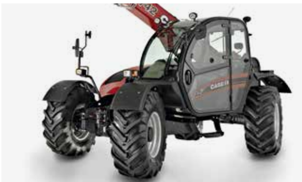
Crab steer: angled driving in a straight line, for working along walls, for example.
