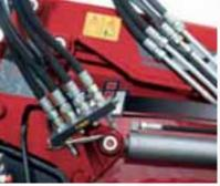
FAST AND EASY CONNECTION Factory fitted: plug & play loader coupling
